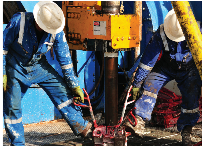
Hand placement: Think about the best placement of your hands to avoid injuries from hazards.
